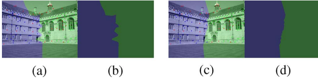
Fig. 5. Closest homography using KNN. First and third columns show, using color tints, the pixels closest to neighbors in consensus attached to a homography, using one- and seven-neighbor methods, respectively. Notice that the images in the Wadham sequence have two major planes and, therefore, two homographies. Second and fourth columns show the tints without the images for clarity. Images were obtained without guided sampling. (a) One-neighbor method. (b) Tint only. (c) Seven-neighbor method. (d) Tint only.
