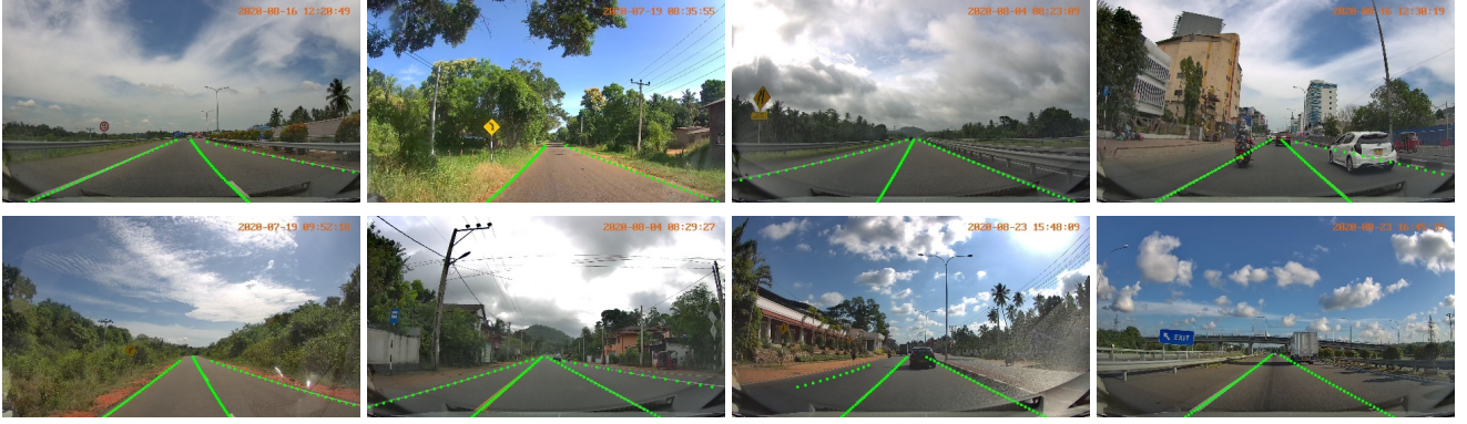
Fig. 5: Visualization of lane detection result on locally captured images. The first six images show accurate detections while the last two show failure cases including false detections and undetected lanes.
