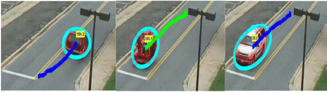
Fig. 6: Trajectories obtained by the EM algorithm for a specific region of interest selected in a VIRAT video clip when vehicles move in isolation. Integer part of the displayed number represents the frame at which the vehicle is detected and the non integer part of the number indicates the assigned cluster number when it is detected. The obtained tracking result is good and is best viewed in color.
