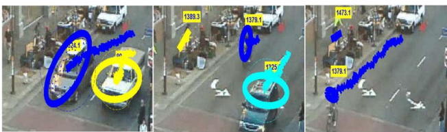
Fig. 7: Trajectories obtained after applying hierarchical clustering to a specific region of interest in Kim's video. The obtained tracking result is satisfactory and is best viewed in color.
