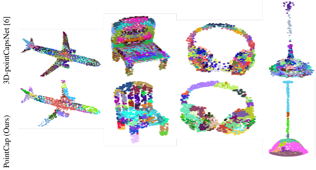
Figure 3: Part representation with dynamic routing in 3D-pointCapsNet [6] (Row 1) and with Euclidean routing in PointCapA (Row 2). 3D-pointCapsNet interprets 32 parts, each having 64 points, whereas PointCaps has 64 parts with different number of points. Note that PointCaps captures spatial relationships to form more human annotated local regions compared to 3D-pointCapsNet [6]
